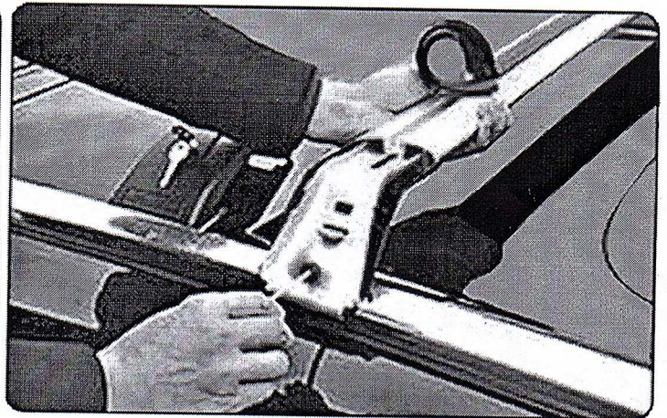
2. Tighten the bar bolts and clamp bolts
